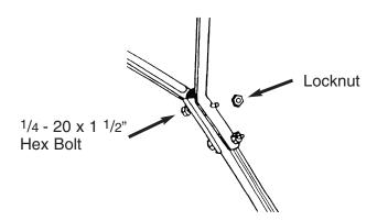
Install control tube between the control tube braces and secure with two 1/4-20 X 1 1/2" hex bolt and locknuts.
