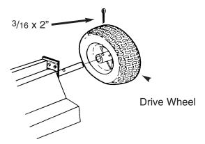
Slide wheels onto each end of axle with the longer portion of the wheel facing the hopper. Secure wheels with 3/16 dia. x 2" cotter pins.
