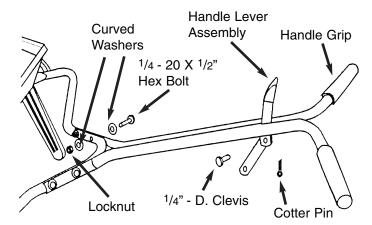
Stand spreader upright on wheels. Attach upper handle assembly to handle brace (make sure handle is positioned as shown) using four 1/4-20 X 1 1/2" hex bolts, eight curved washers, and four locknuts. Tighten securely. Install handle grips onto upper handle. Slide handle lever assembly between handle brackets and secure with 1/4 diameter clevis and cotter pin. Make sure lever pivots freely.
