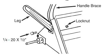
Remove spreader and components from carton. Place hopper on its front panel, insert two 1/4-20 X 1/2" hex head bolts through the leg; flattened end of handle brace and holes in hopper as shown.
