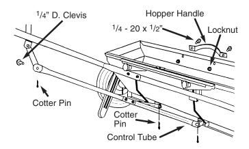
Slide the ends of the control tube braces over the studs on the shutoff bar brackets; secure with cotter pins. Attach opposite end of control tube to the handle lever using 1/4 diameter clevis and cotter pin. Make sure handle lever operates freely. **Tighten all Nuts left loose in Step #1.** Install hopper handle on front of spreader using two 1/4-20 X 1/2" hex bolts and locknuts.
